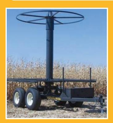
The **Stringer Trailer** provides reliable, convenient transport of tile to and in the field.
