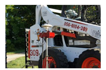
GPS L1/L2, Glonass G1/G2, BDS B1/B2. Internal radio, External radio, or Ethernet, or any combination. The choice is yours, built for you, by AgRePlan.
